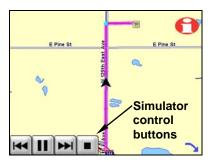
The red X on the GPS Simulator button (left) indicates the feature is turned off. The unit simulating a route is shown at right. The simulator control buttons are located in the bottom left corner of the map screen.
